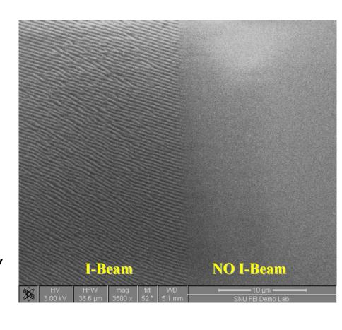
Fluence range, 10<sup>13</sup>~10<sup>16</sup> ions/cm<sup>2</sup>, controlled by the current, exposing time and exposing area
